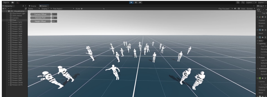
Figure 2: Thirty connected simulated dancers, generated using prerecorded motion signals transmitted among DanceGraph clients, the signals being simulated are indistinguishable from those generated in real-time by live ZED camera captured dancers.
